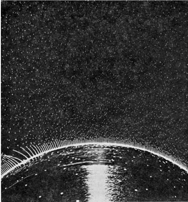
Fig. 1. Contact print (without enlargement) showing cusps and atomization near edge of 4 in. bell at 900 rpm, delivery rate of paint 100 cc./min., 100 kv.; good atomization (fine particle size).
